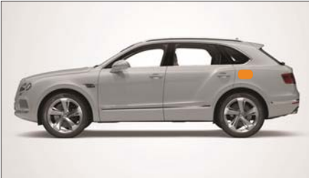
Vehicle charging connection behind the charging socket lid on the left hand rear of the vehicle
