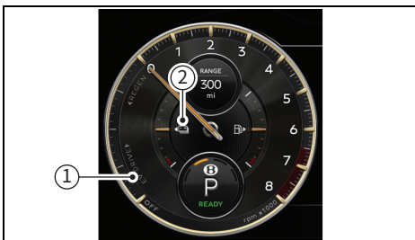
"EV DRIVE" (1) and High-Voltage battery gauge (2) on the instrument cluster
